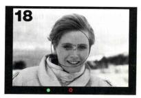
Confirm the green focus indicator LED and the red exposure indicator LED olight up.
