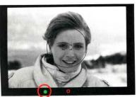
4. Keeping the shutter release button lightly pressed, watch the focus indicator LED in the viewfinder and rotate the lens focusing ring manually until the focus indicator LED lights up.
